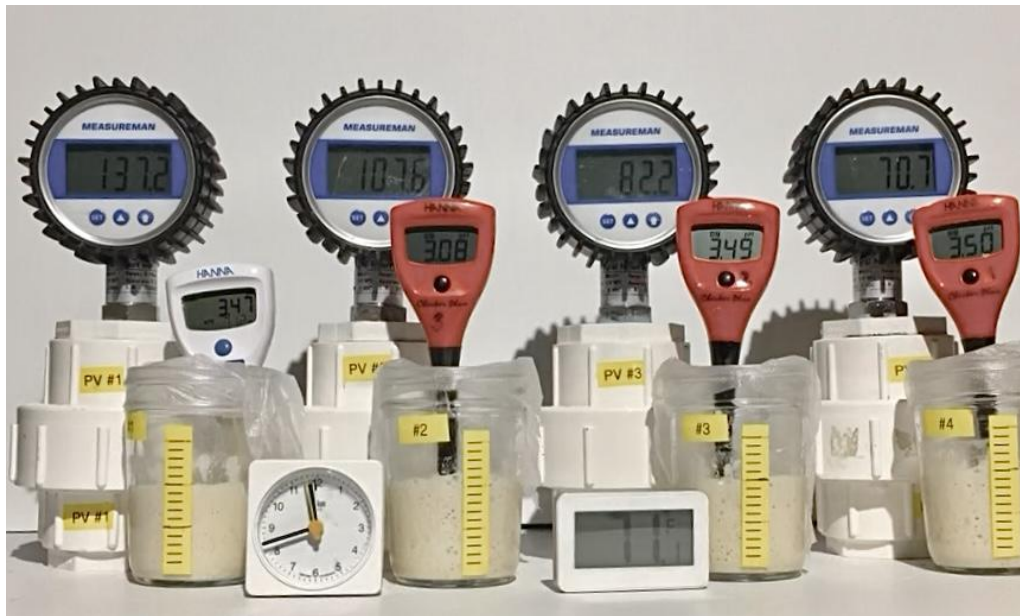
Four-vessel sourdough starter CO 2 testing apparatus. Digital pressure gauges measure CO 2 accumulation in sealed vessels under controlled experimental conditions, with parallel open-air samples used to measure visible attributes and pH.
